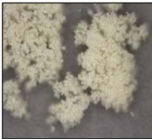
Figure 3: sulphur sediment (magnified \*10).
